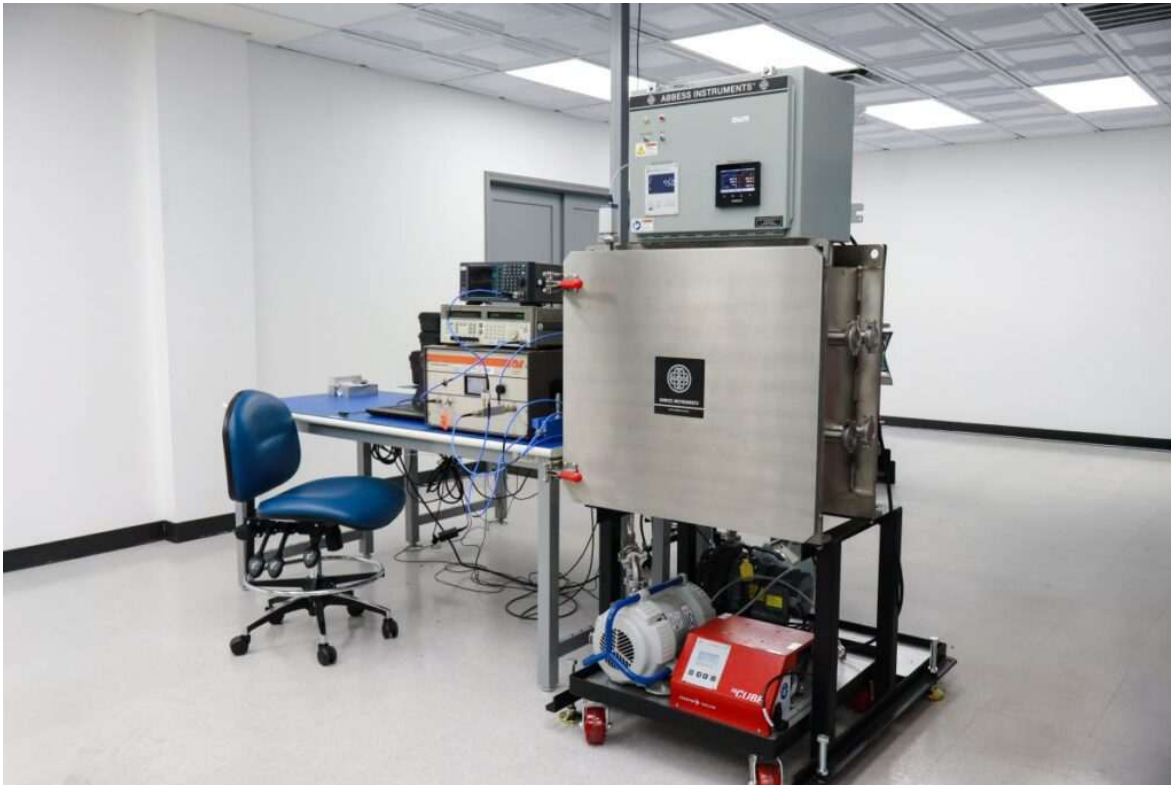
Figure 3 – High Power RF testing in a hypobaric chamber
