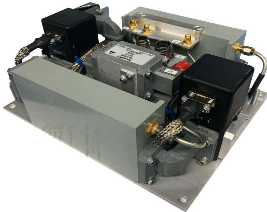
Figure 1 – Example of an integrated Ku-band TX/RX microwave assembly
