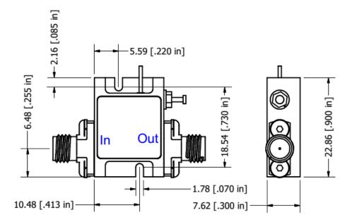
Field replaceable SMA Connectors
